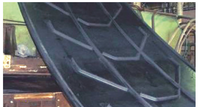
Figure 2: chevron profile of the belt obtained by mold
