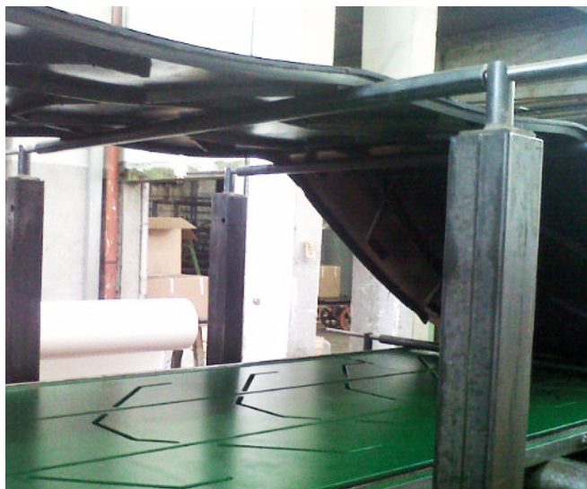
Figure 1: metal mold used to obtain the chevron profile and the guides on the belt
