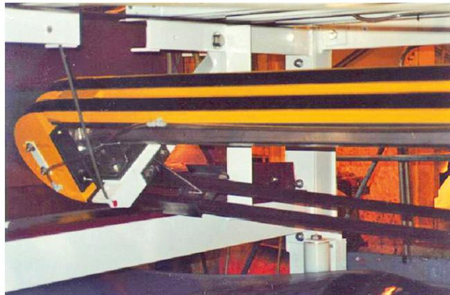
*Wear belts mounted on a vacuum box - FLSMIDTH Italy courtesy*
