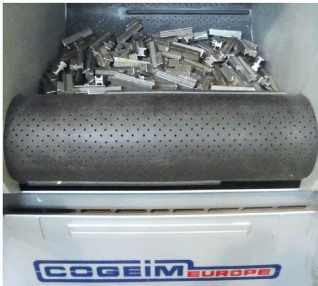
GRITROLL belts are used on Shot and Sand-blasting machines, usually for finishing small parts loaded in bulk and, in its cradle-configuration, it gets the parts to be worked and keep them in continuous tumble.
